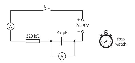
(a) Describe how the results of this experiment are obtained **and** used to show how the voltage across the capacitor varies with time while the capacitor is charging.
