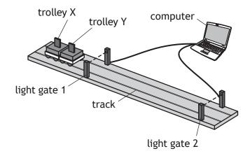
The trolleys X and Y are moving together to the right at  $0.40 \text{ m s}^{-1}$ .
