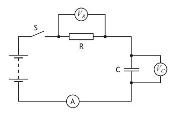
The capacitor is initially uncharged. Switch S is closed.
