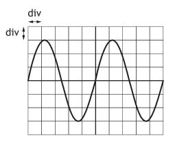
The Y-gain setting on the oscilloscope is 2.0 V/div.
