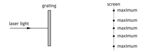
A series of interference maxima are observed on the screen.
