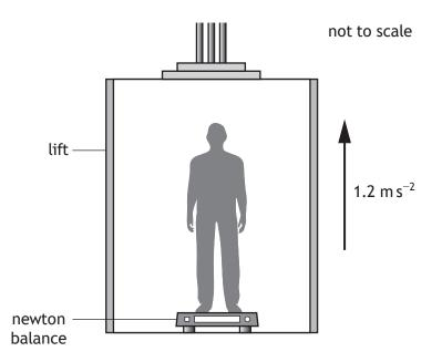
The mass of the student is 50.0 kg. The lift accelerates upwards at  $1.2 \text{ m s}^{-2}$ . The reading on the newton balance is:
