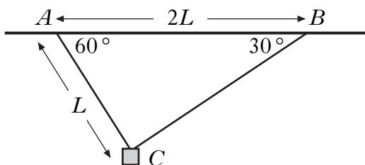
The distance between  $A$  and  $B$  is  $2L$  metres and the string  $AC$  has length  $L$  metres.
