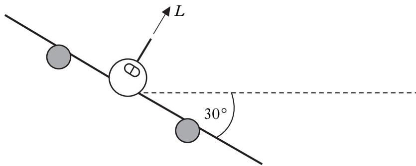
The wings of the aircraft are banked at  $30^\circ$  to the horizontal and generate a lift force of  $L$  newtons. This force acts perpendicular to the wing surface, as shown in the diagram.
